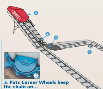
Large, double-flanged, 12" (305 mm) corner wheels are designed to contact only the back of the link. The wheel is through-hardened to a specific hardness that resists wear. Each corner wheel has a greasable composite bearing.
